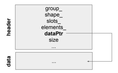
For ArrayBuffers with size <= 0x60 bytes, data is located inline right after the header.
